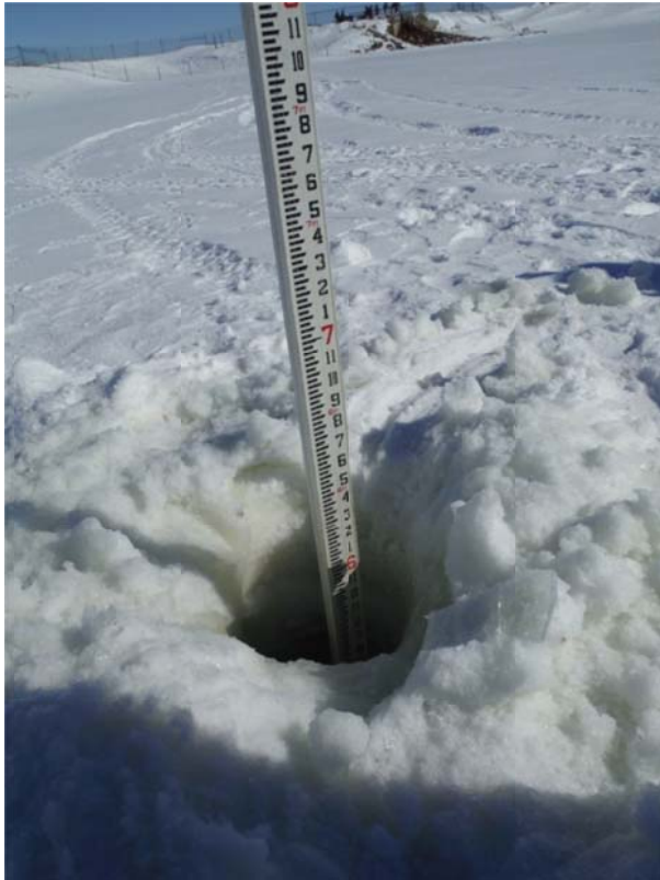
Measuring depth of ice, depth of water, and elevation of lagoon bottom (or berm wall).
