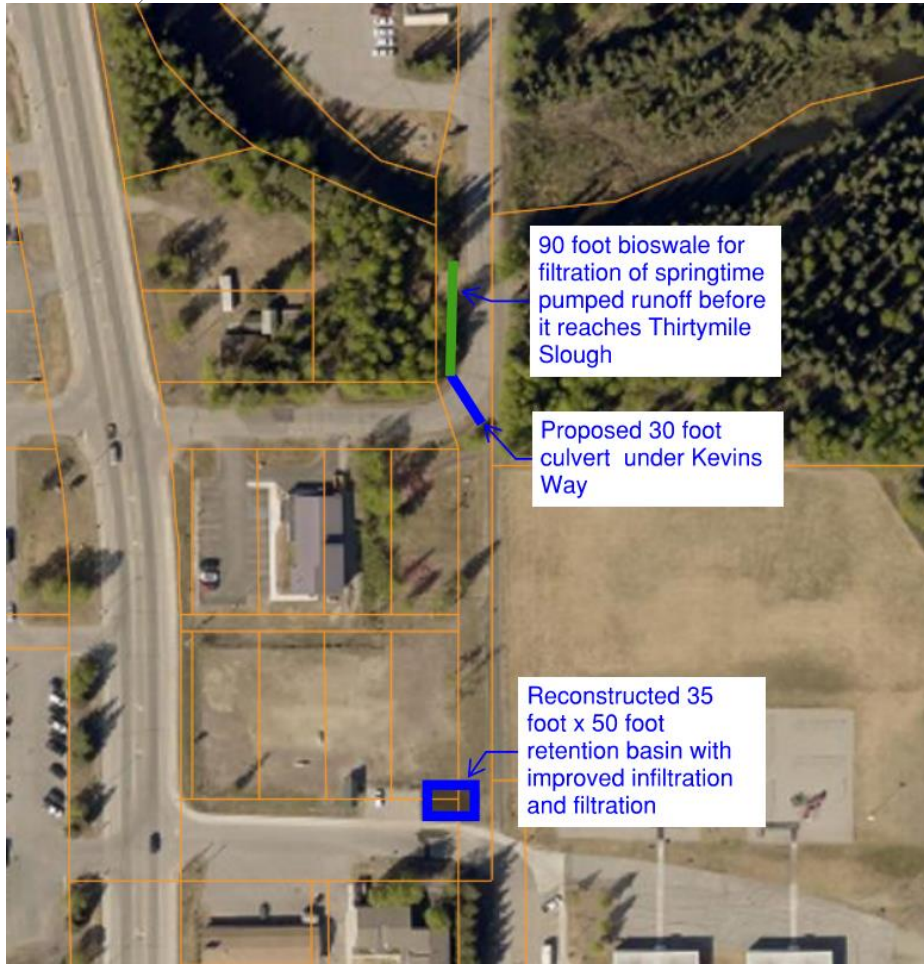
Image 1: Proposed culvert under Kevins Way/Snowman Lane curve and bioswale in the right-of-way to the west of Snowman Lane
