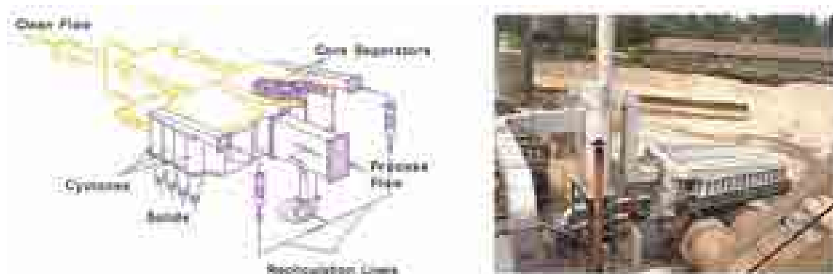
Figure 4-6. Schematic (left) and actual (right) core separator system [EPA, 2003]
