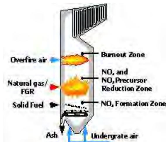
Figure 2-2. Gas reburn applied to a stoker boiler [www.gastechnology.org]
