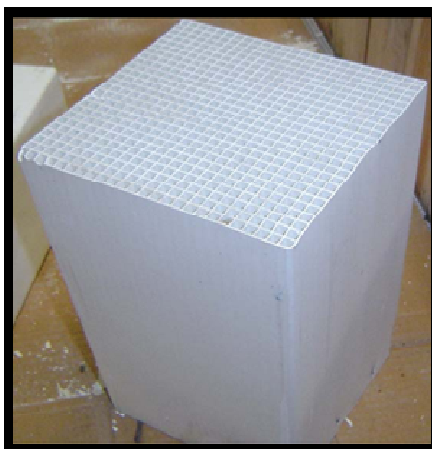
Figure 2-6. Block of monolith ceramic heat exchanger [Toupin, 2007]
