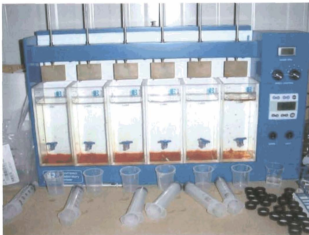
Figure 6 – Jar test with \text{KMnO}_4 , followed by 80/20 blend of SternPAC and Arctic Floc 12100
