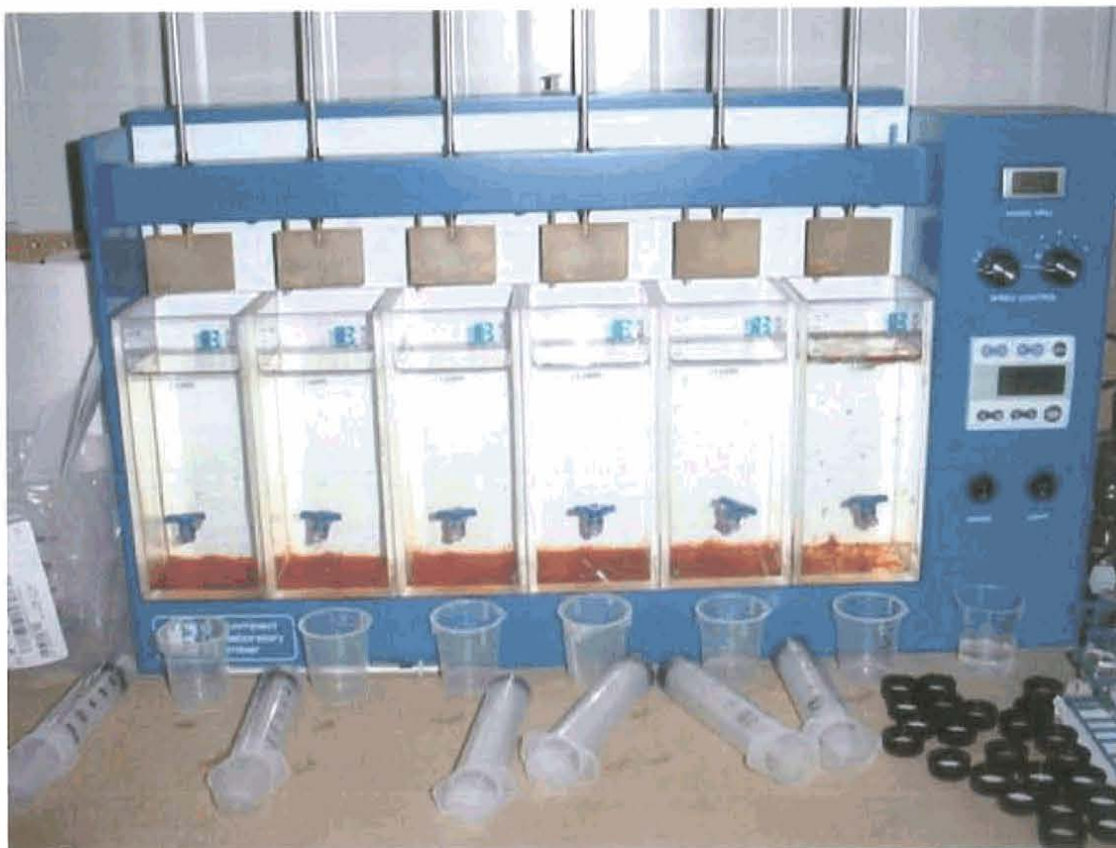
Clear water after a successful jar test. Sludge in bottom of jars contains iron, manganese, arsenic, and removed color compounds.
