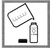
**2.** Fill a round sample cell with 10 mL of sample.
