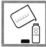
**6.** When the timer beeps, fill a sample cell with at least 10 mL of sample (this is the blank).
