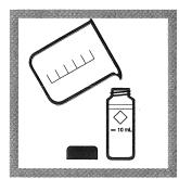
**5.** When the timer beeps, fill a second sample cell with 10 mL of sample (this is the blank).
