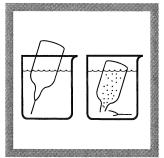
**3.** Fill a NitriVer 3 Nitrite AccuVac® Ampul with sample. Keep the tip immersed while the ampule fills.
