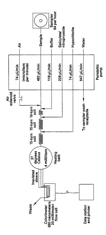
Figure 3.—Nitrogen, ammonia, low ionic-strength water, salicylate-hypochlorite manifold.
