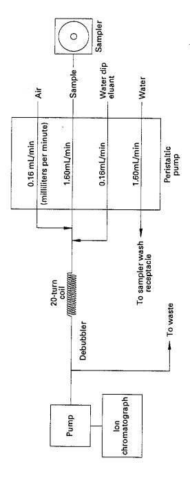
Figure 1.—lon chromatography matrix matching manifold.
