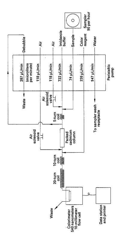
Figure 8.—Nitrogen, nitrite plus nitrate, cadmium reduction-diazotization manifold.
