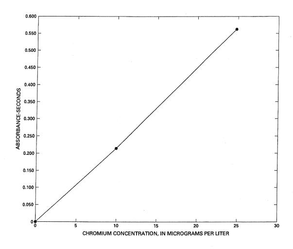
Figure 2.—Typical calibration curve for the determination of chromium by graphite furnace atomic absorption spectrophotometry.
