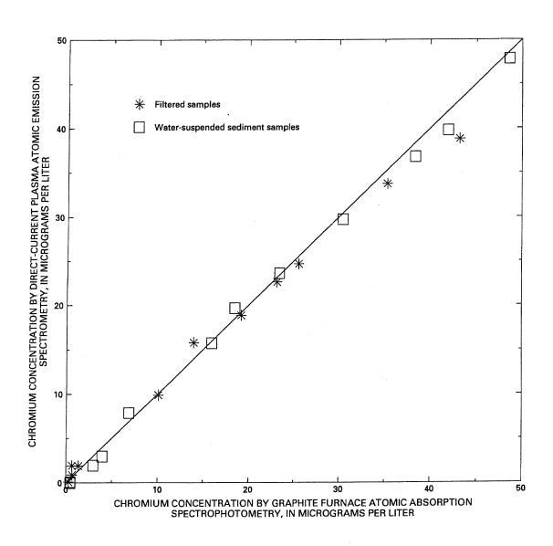
Figure 3.—Analytical results for the determination of chromium by direct-current plasma atomic emission spectrometry and graphite furnace atomic absorption spectrophotometry.
