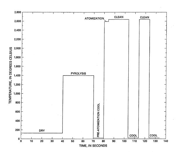
Figure 1.—Time, temperature, and function of the graphite furnace atomic absorption spectrophotometry program when using a heated graphite analyzer.
