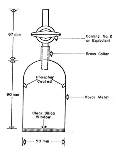
Figure 3. A typical scintillation cell for radon counting
