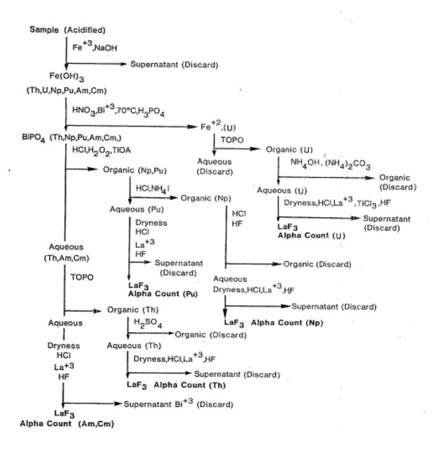
Figure 6. Generalized chemical procedure (for actinide elements)
