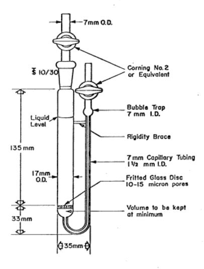
Figure 2. A typical radon bubbler
