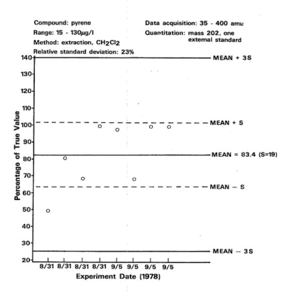
Figure 2. Control chart for pyrene in reagent water.
