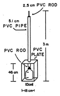
Figure 3 - Jar Sampling Device
