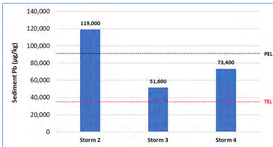
Figure 3-5. Wet weather lead sediment sampling at the east outfall 2011–2012 (Davis et al., 2013a)
