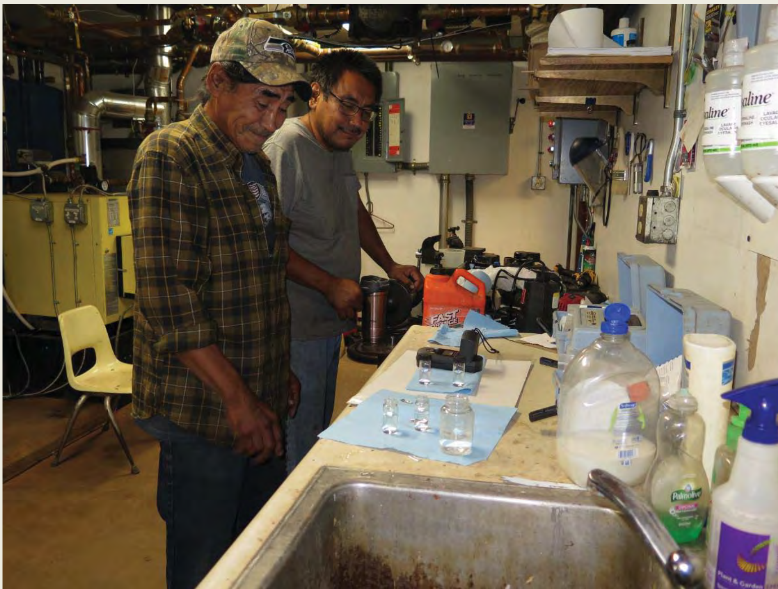
Photo 48: Primary operator Paul Petruska and backup Aaron Petruska demonstrate use of the Hach Pocket Colorimeters for chlorine, iron, and manganese.
