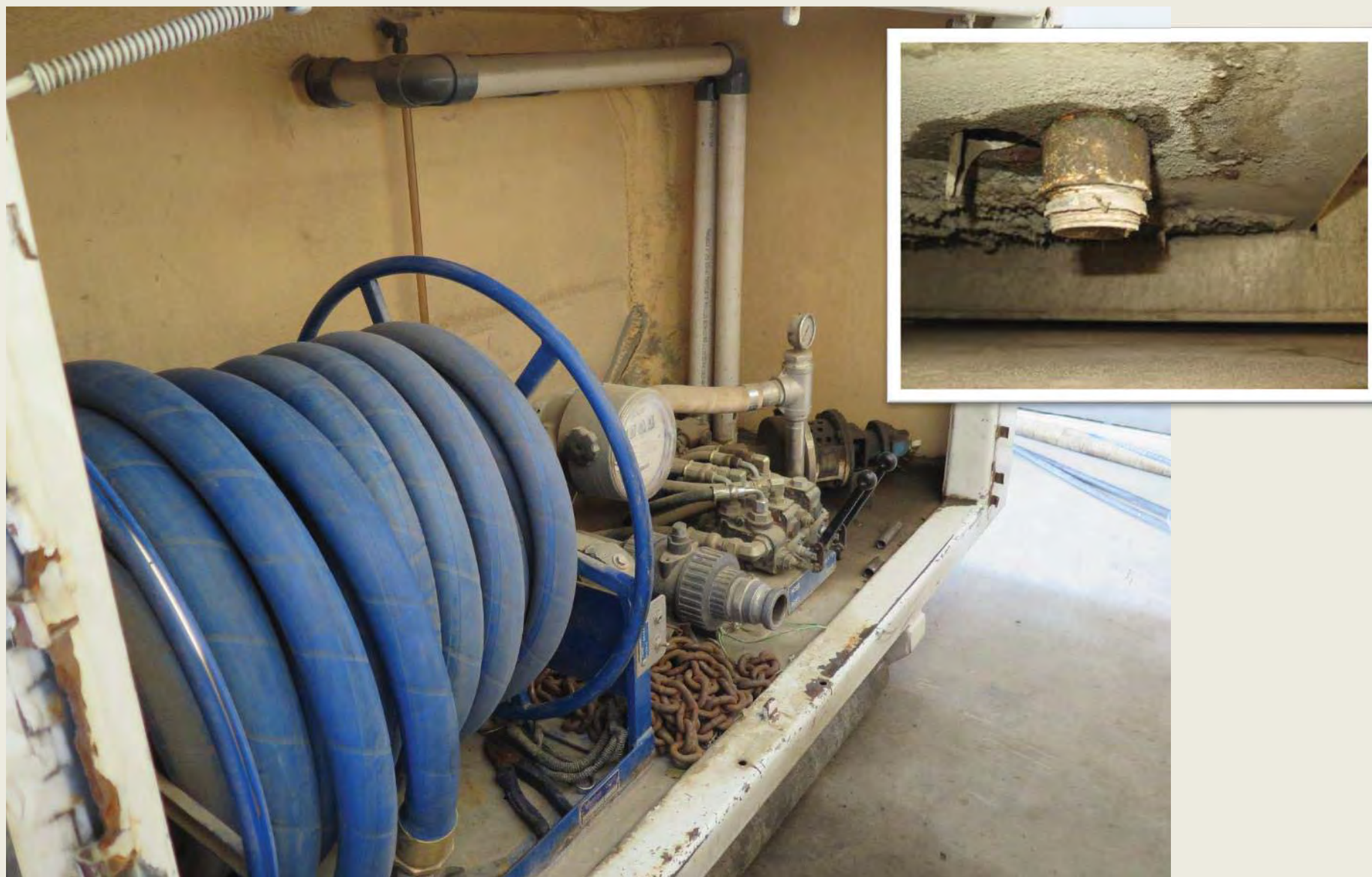
Photo 45: Water haul tank pump, meter, and fill hose. Tank overflow/vent piping coming from top (outlets shown in inset image)
