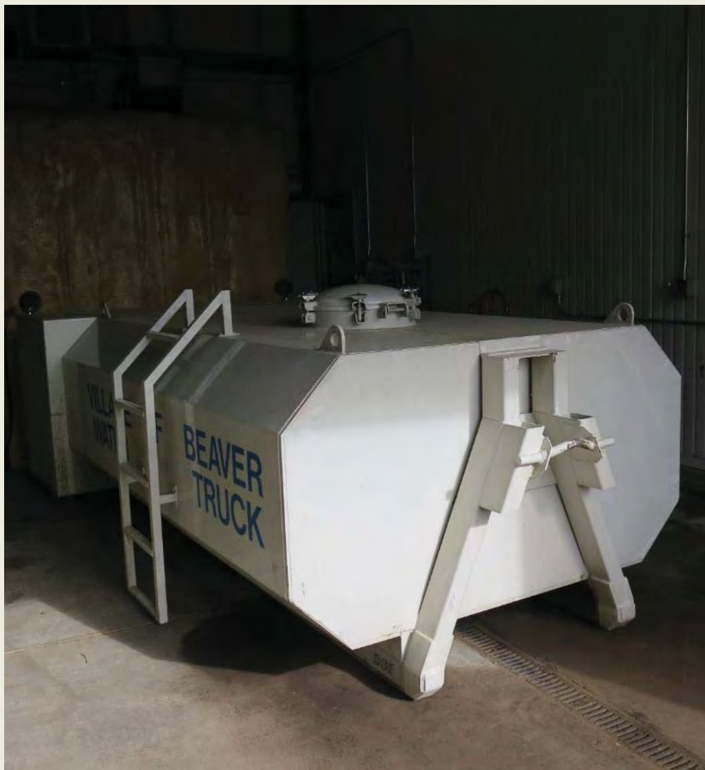
Photo 44: Haul truck with sewage tank on back; water tank stored in separate garage. Water tank is separate and installed with hook/hoist when delivering water.
