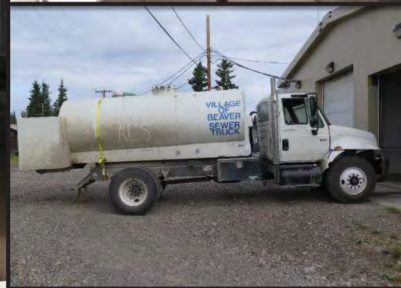
Photo 44: Haul truck with sewage tank on back; water tank stored in separate garage. Water tank is separate and installed with hook/hoist when delivering water.
