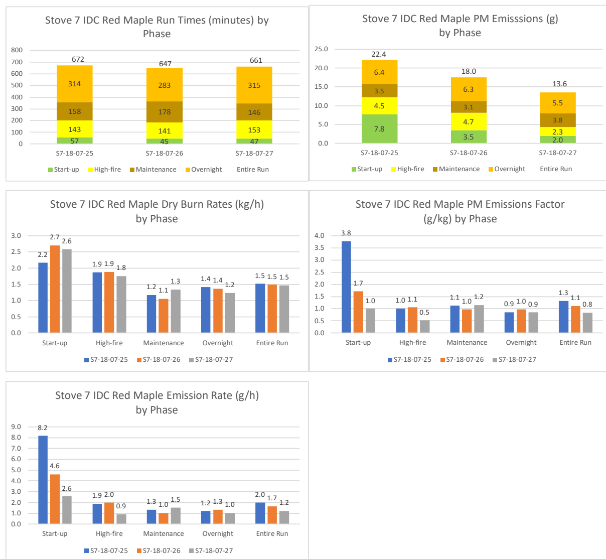
Figure 124. Stove 7—IDC Red Maple Run Parameters
