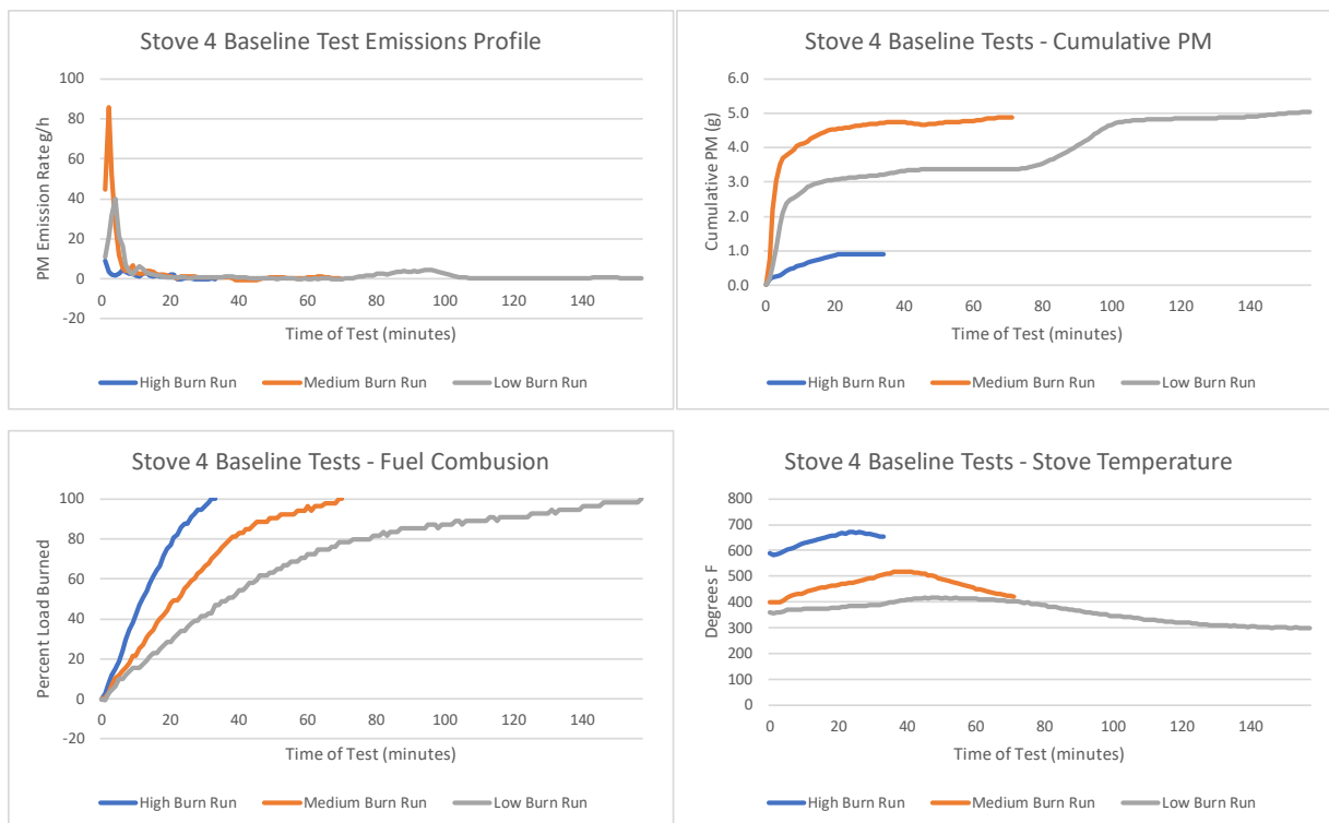
Figure 20. Stove 4—Baseline Runs—PM Emission Profiles, Cumulative PM Emissions, Cumulative Fuel Consumption, and Stack Temperatures
