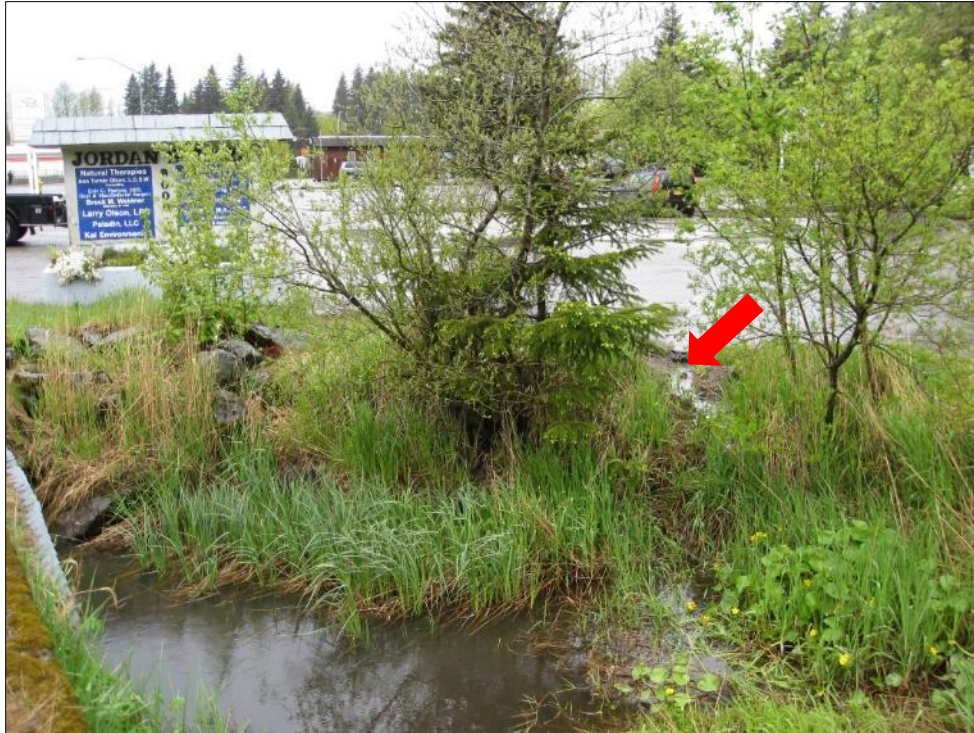
Figure 43. Runoff from a parking area on the south side of the Jordan Square North parcel flows through a narrow strip of vegetation before entering Jordan Creek. View looking west in May 2015.
