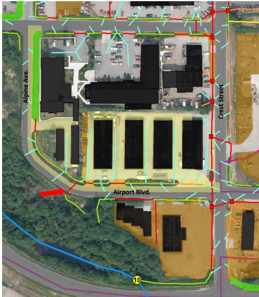
Figure 55. The Alpine Ave. South – Airport Blvd. West stormwater system. The contributing area is shown in yellow; red arrow indicates the outfall pipe.
