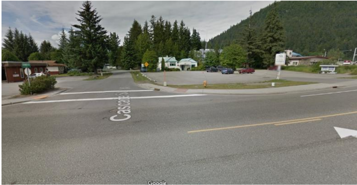
Figure 22. Google Street View of the north side of Glacier Hwy. at Cascade Street in July 2020. Parking lot and highway runoff could be conveyed into stormwater BMPs constructed in existing grass-covered (photo-right near hydrant) and landscaped (photo-left near stop sign) areas on private parcels that abut the roadways.
