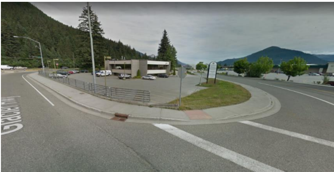
Figure 20. Google Street View of the intersection of Old Dairy Road (right) and Glacier Hwy. (left) in July 2011 (view looking east). Highway runoff could be directed from the curb and gutter to a stormwater BMP constructed in the grass-covered area in the Old Dairy Road right-of-way.
