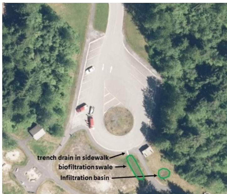
Figure 12. A stormwater BMP next to Eagle River in the Eagle Beach State Recreation Area in Juneau. Runoff flows from the parking lot to a biofiltration swale through a trench drain in the sidewalk. Runoff exiting the swale flows through a buried culvert (not depicted above) into an infiltration basin.
