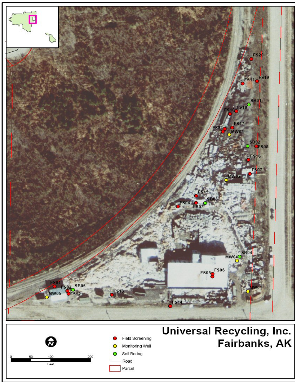
Figure 4-1 Locations of Field Screening, Soil Borings, and Monitoring Wells
