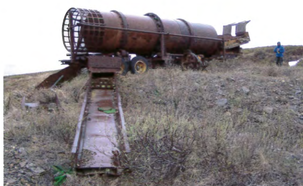
4. Roller mill with sluice line intact.
