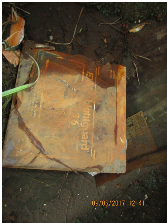
Photo 18: Loose lead-acid battery laying on ground next to building.
