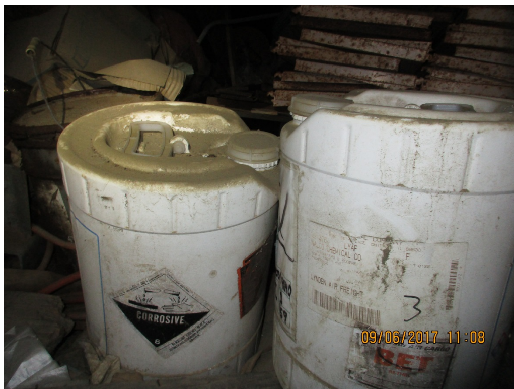
Photo 23: Loose containers of corrosive chemicals under building.
