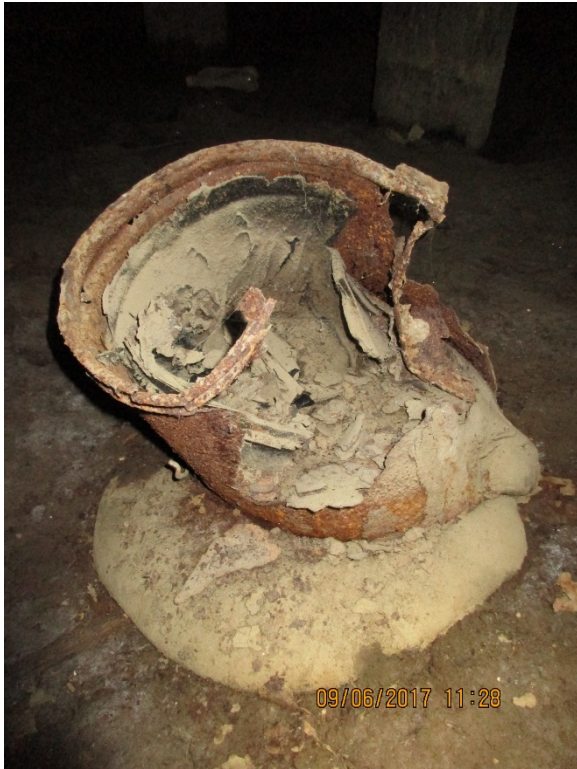
Photo 11: Loose 5-gallon bucket of asbestos-containing roof patching tar under building.
