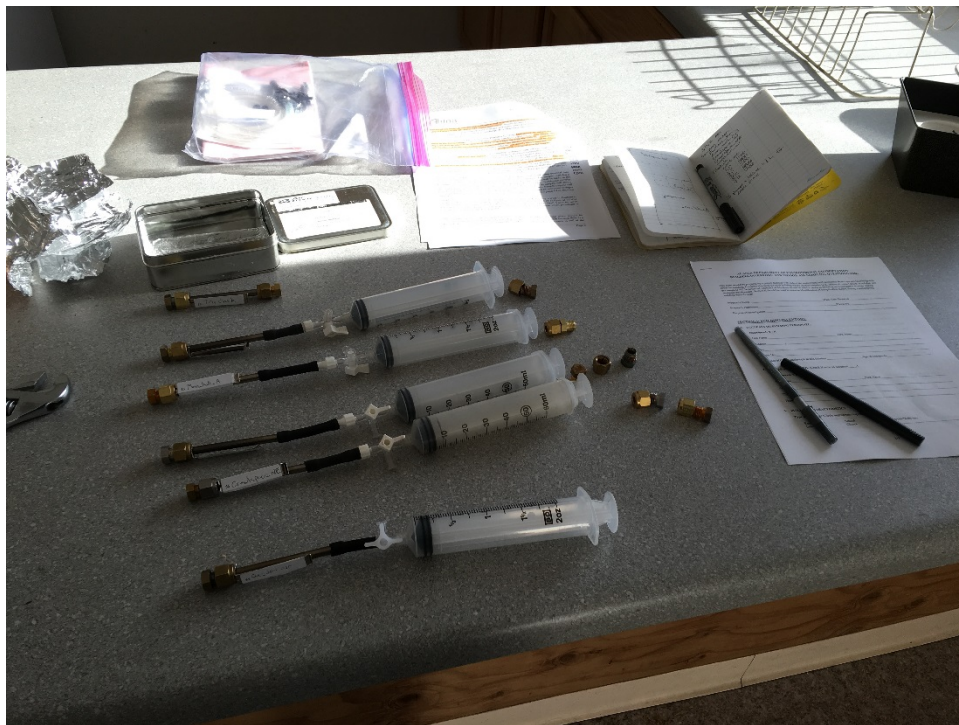
Photo 35 – Preparing TO-17 tubes for air sampling
