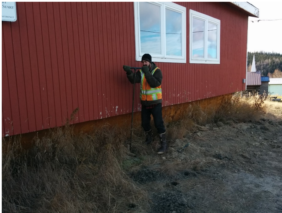
Photo 21 – Hand-auguring SB-16 between UST and building
