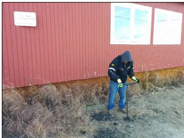
FIGURE 11 – HAND AUGURING SOIL BORINGS NEAR UST
