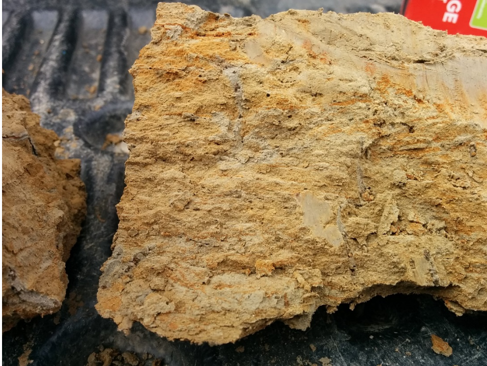
Photo 17 – Silt clump from test pit TP-02
