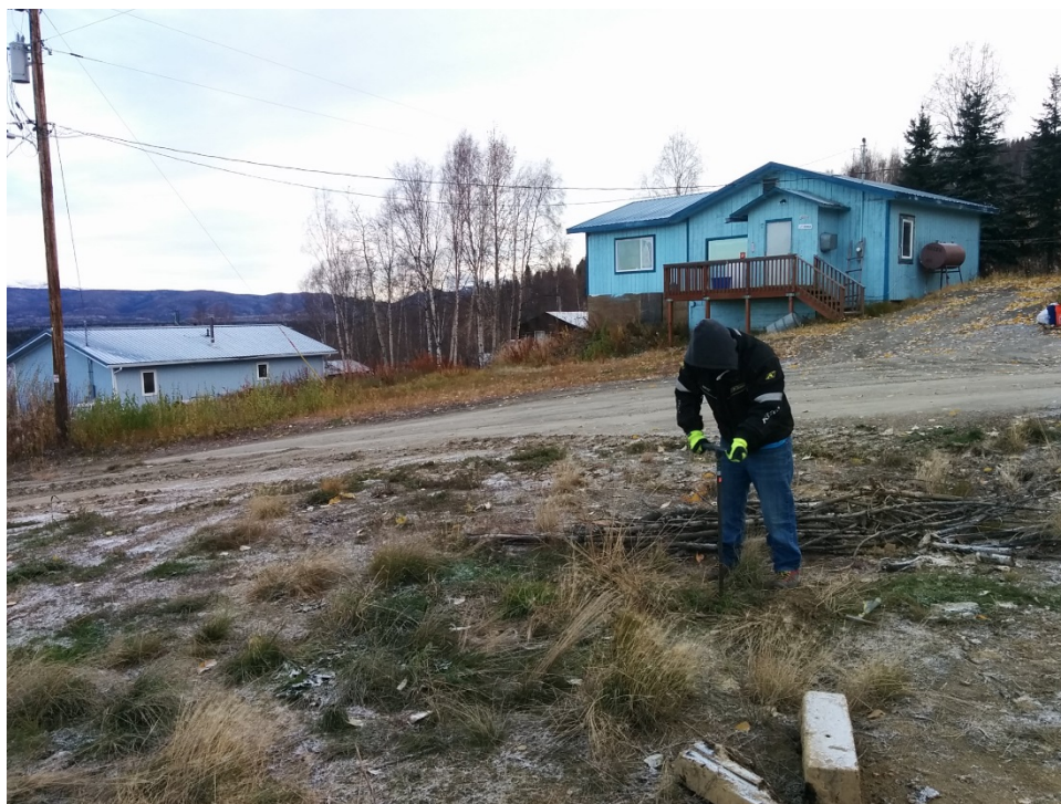
Photo 20 – Hand-auguring soil borings in former AST area
