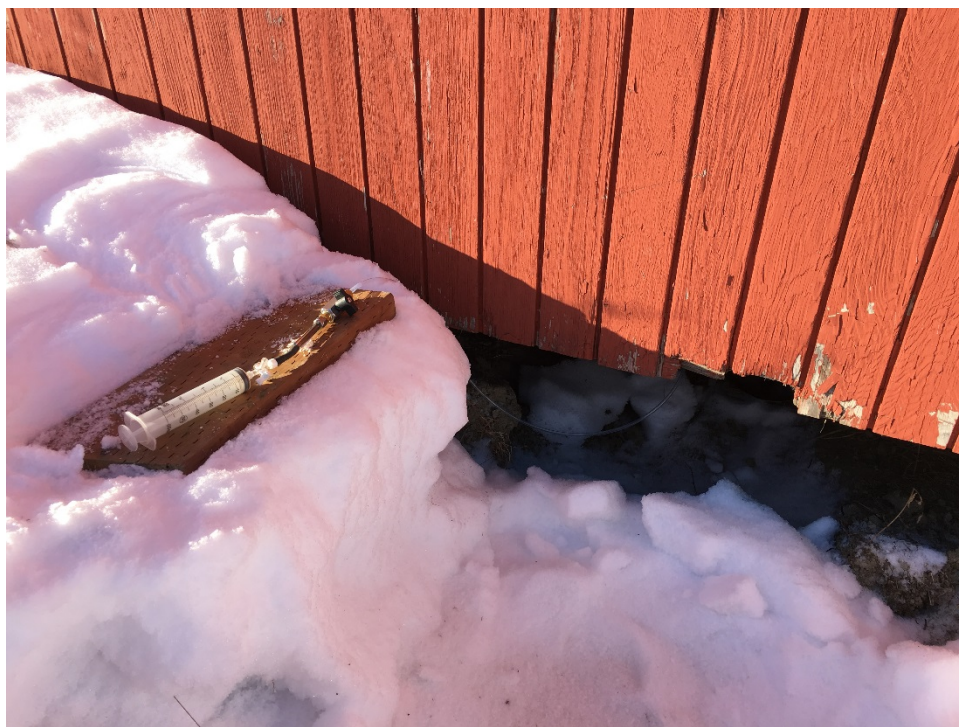
Photo 38 – Tubing rigged up to sampler for crawlspace air sampling
