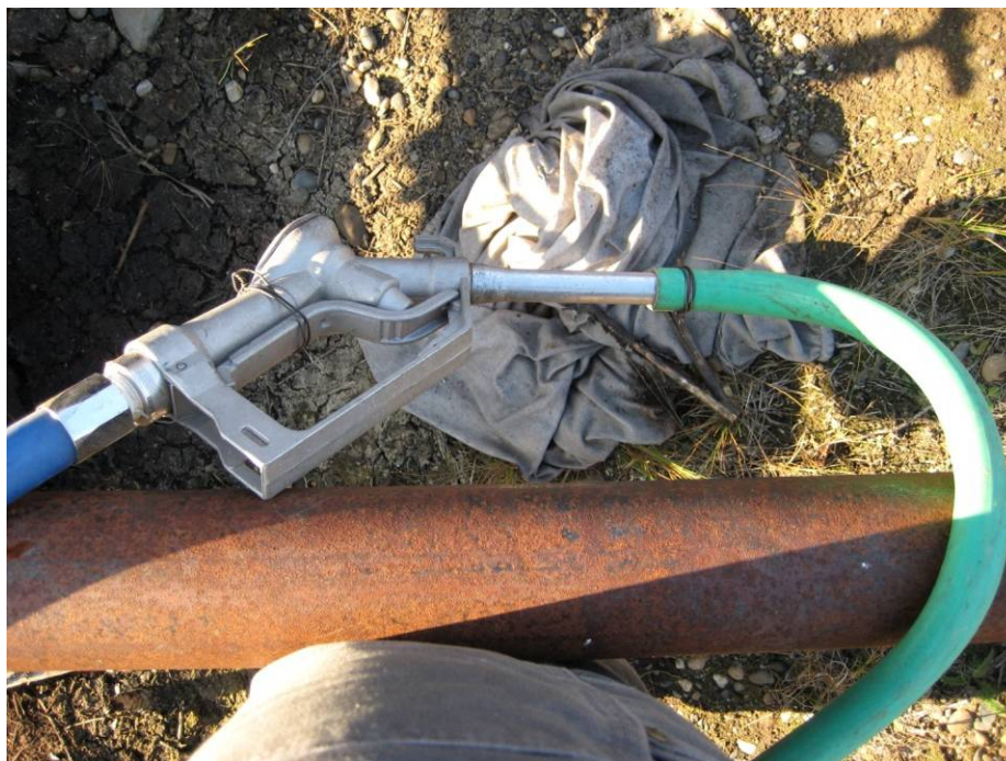
Photograph 4: Fuel pump with garden hose used for fuel line (September 2009).
