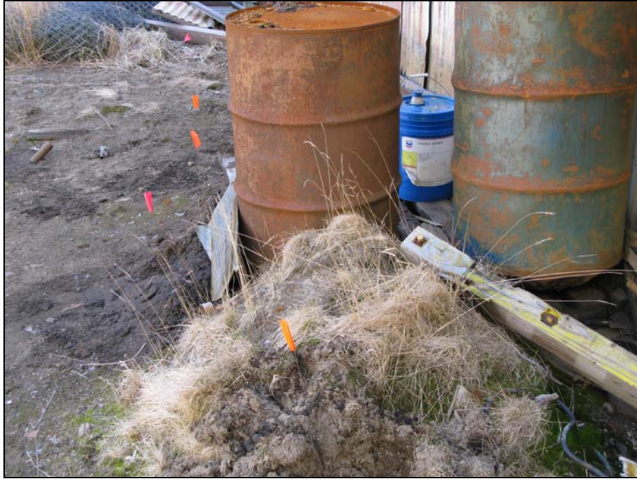
PHOTOGRAPH 1. TWO 55-GALLON DRUMS AND ONE 5-GALLON BUCKET PARTIALLY FILLED WITH OIL LOCATED BETWEEN BUILDINGS F AND H. RED FLAGS SHOW LOCATIONS OF SOIL SAMPLES.
