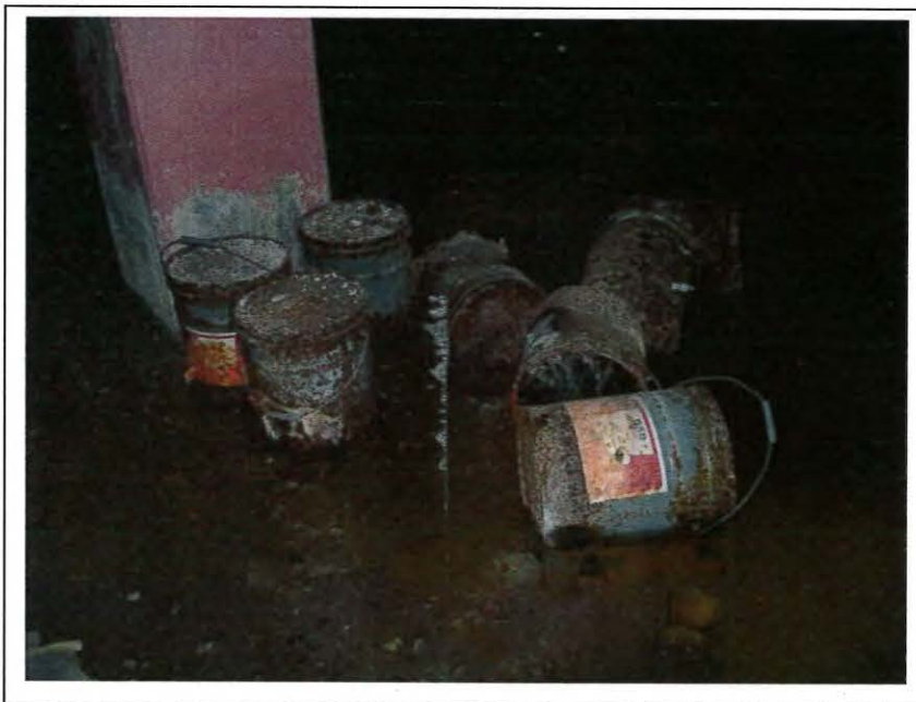
Photo H-24: Five-gallon buckets of the adhesive "DAP." Note the buckets were full of a solid black material. (September 8, 2014)
