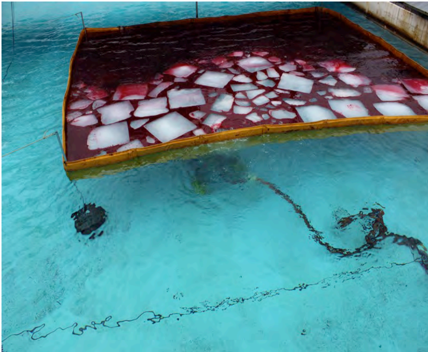
Ohmsett Testing in Feb 2016 Ice Coverage at 30% with Oil
