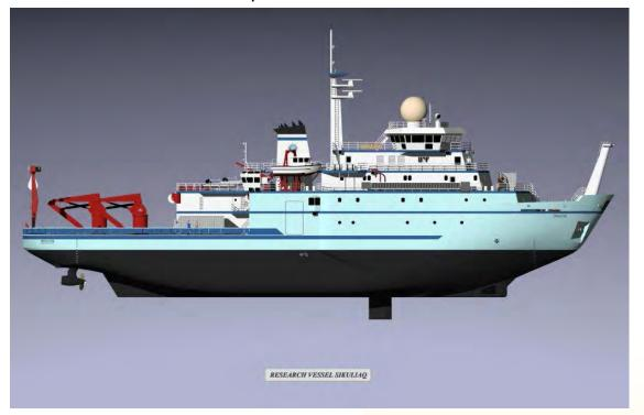
The SIKULIAQ allows researchers to collect sediment samples directly from the seafloor, hosts remotely operated vehicles, uses a flexible suite of winches to raise and lower scientific equipment, and conducts surveys throughout the water column and sea bottom using an extensive set of research instrumentation.
