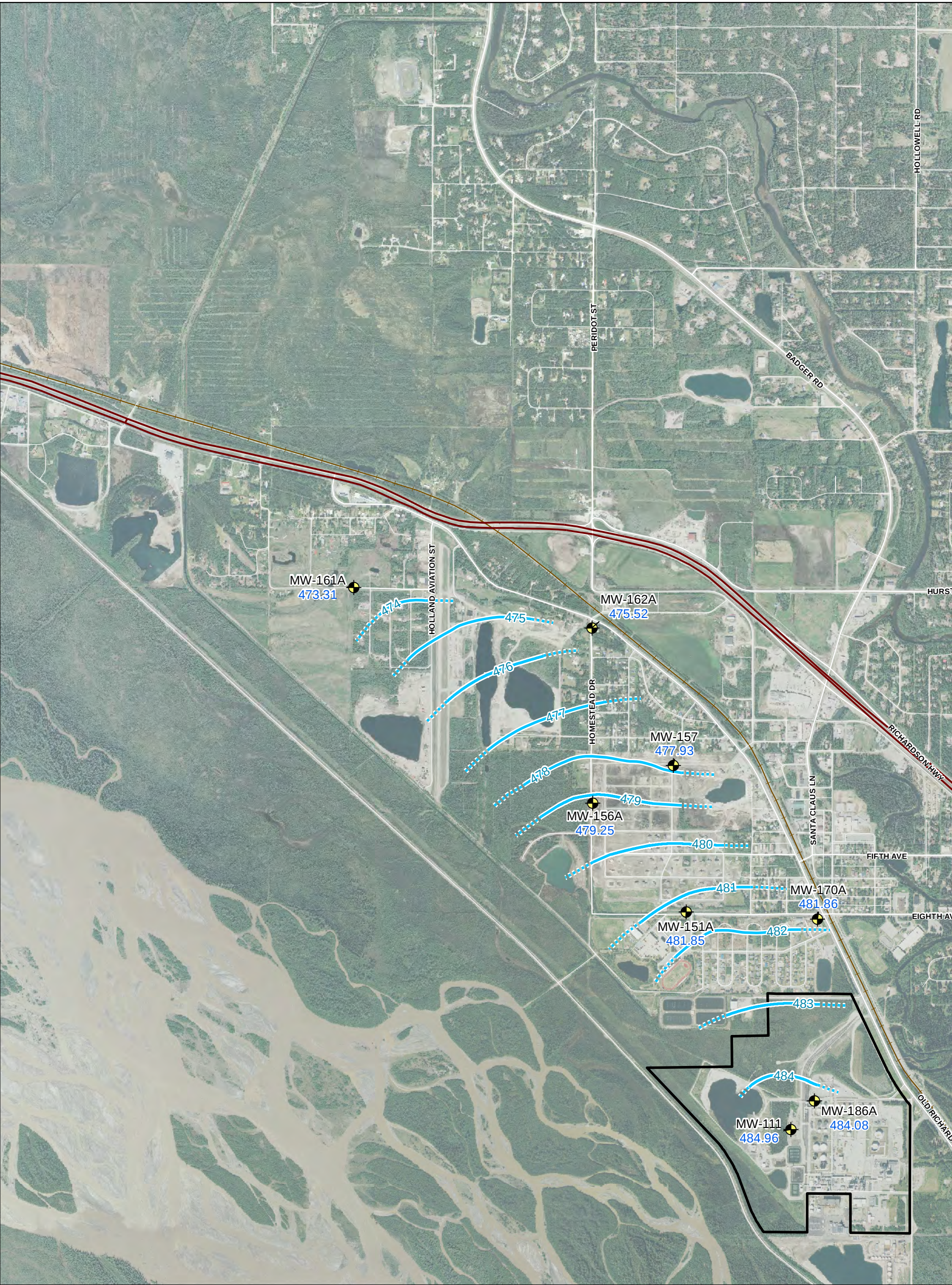
Figure 52 GROUNDWATER ELEVATIONS AT THE WATER TABLE MARCH 11, 2011 DATA LOGGER MEASUREMENTS North Pole Refinery Flint Hills Resources Alaska, LLC
