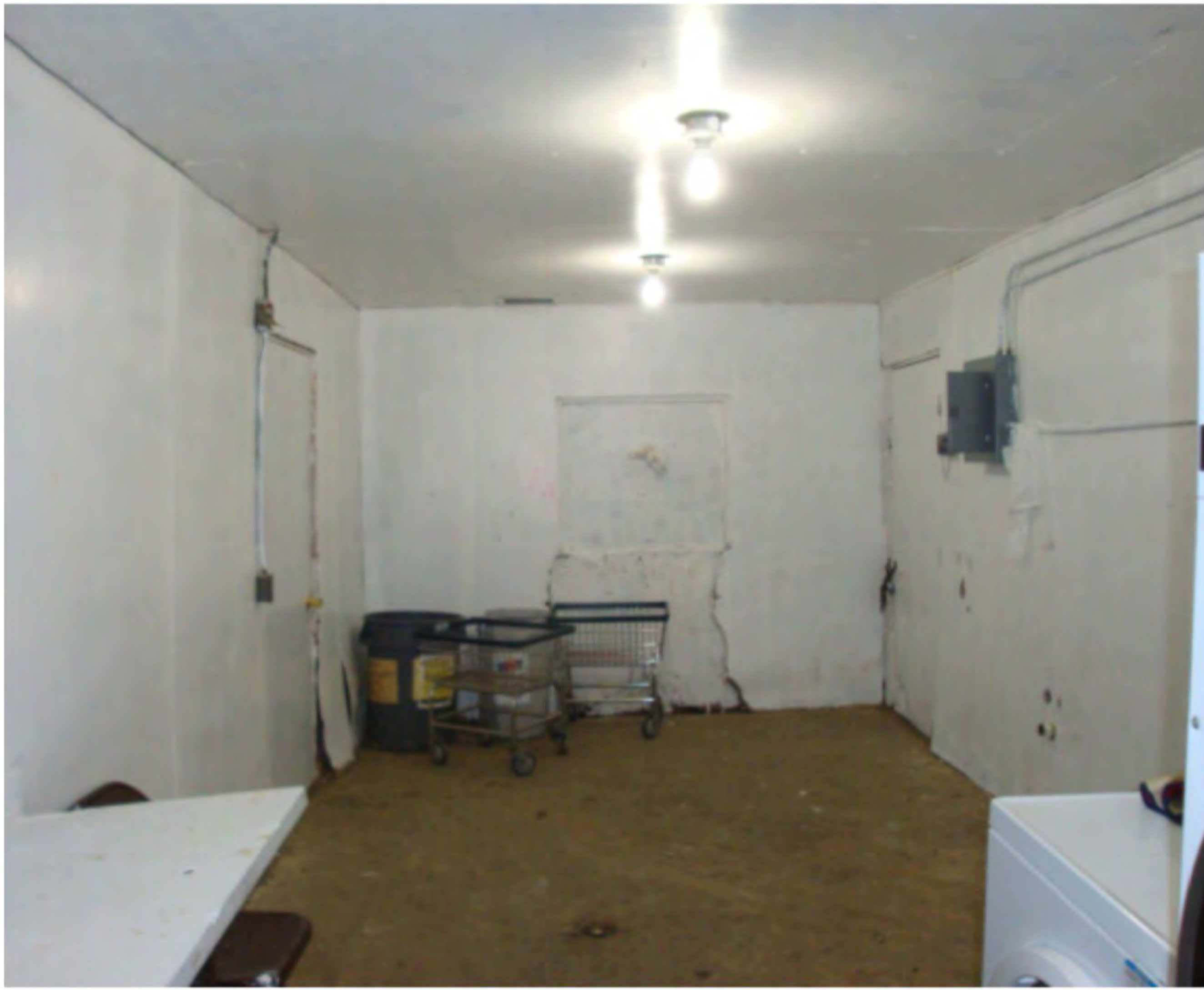
Tununak Washeteria. Photo shows decay of the door and flooring, and peeling of the wall.
