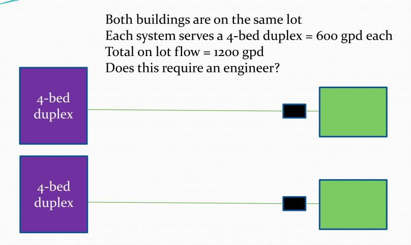
Can be installed by a Certified Installer Each system serves a single "multi-family" dwelling and the total flow for the lot is less than 1500 gpd.
