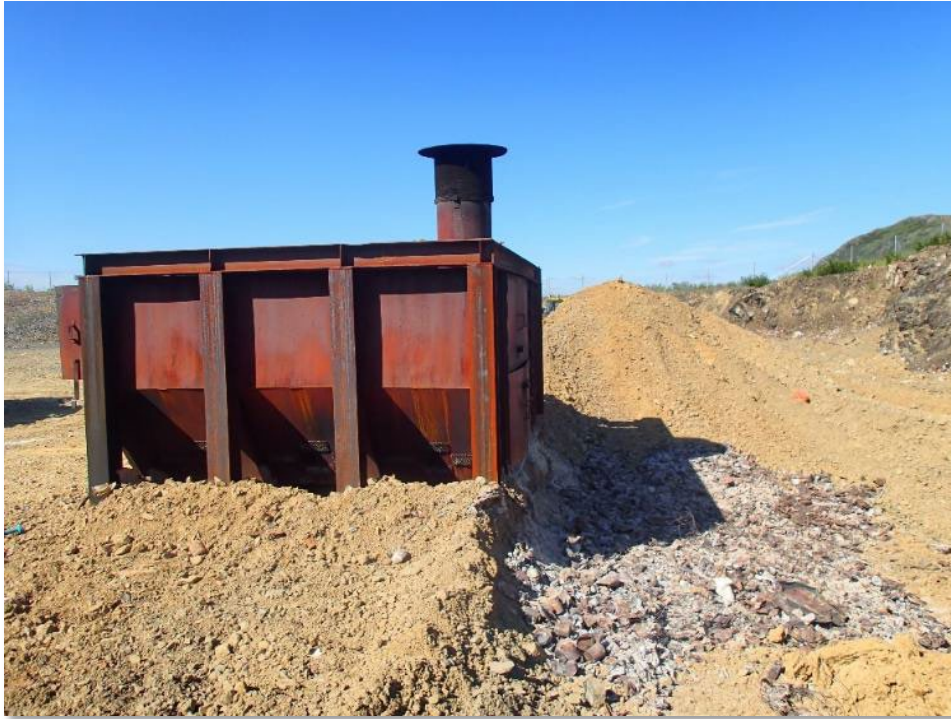
Enclosed commercial burn unit.
