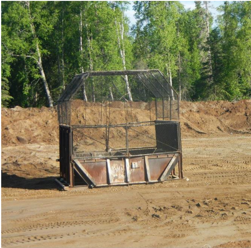
Commercial burn unit.
