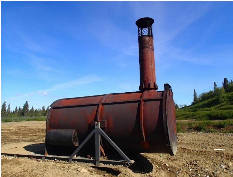
Enclosed commercial burn unit.
