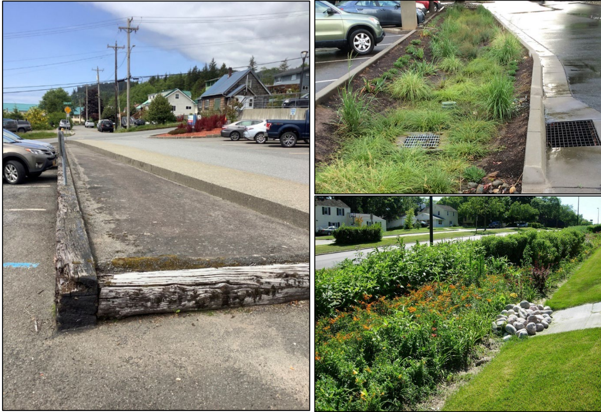
Figure B.5. Left: Unused paved area in office complex parking lot on Carlanna Lake Rd. that could be converted to an infiltration basin or bioswale to capture and treat stormwater runoff from the upper parking lot and/or part of the lower lot. Top right: Example of an infiltration basin that accepts parking lot runoff via curb cuts. Bottom right: Example of a bioretention cell (SWMM LID Controls).
