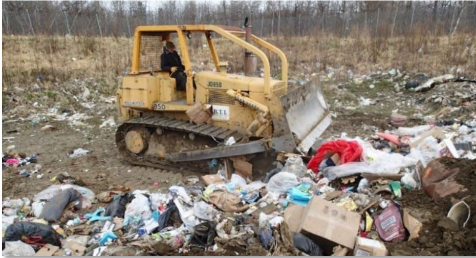
Operator using a dozer to consolidate waste.
